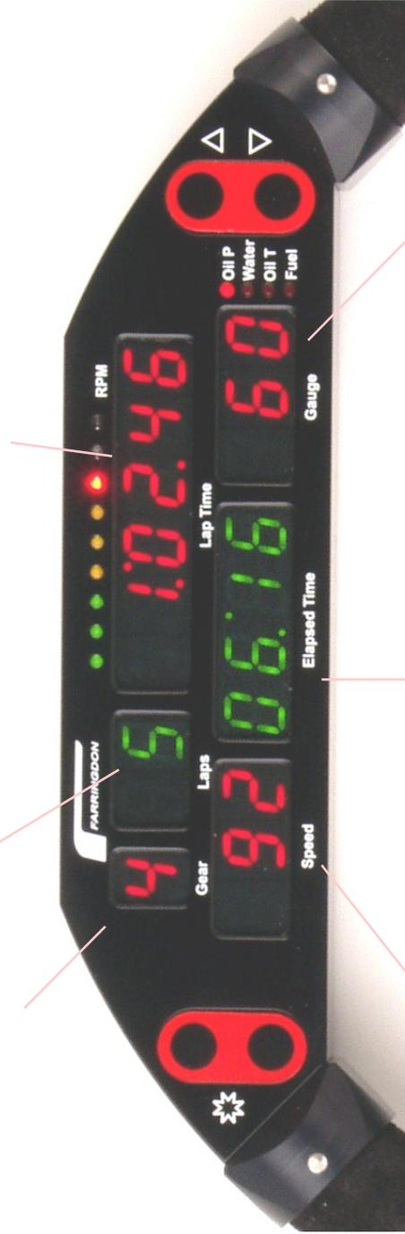
The Speed window can display speed oil pressure, water temperature or oil temperature. If speed is not shown here normally, it can be shown by pressing the top left hand button for 3 seconds—useful for the pit lane. The original display can be restored by pressing the bottom left hand button.
