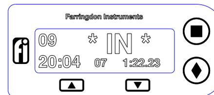
The display will return to Timing Mode when the next Beacon set to the Main Channel is seen. If the IN command from the Beacon is received during the Hold Time, it is not considered as an of lap beacon. (See section 5.)
