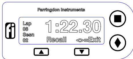
The display shows the last lap recorded. The **▲** button will select the previous lap and the **▼** button will retrieve the next lap. The display will not change if you try to display a lap after the last or one before the first. Note that the session number is displayed as well. To make the Recall (and the Up Load) mode more useful, it is worthwhile changing the session number every time the system is switched on and recording the details of the new session - car set up etc..
