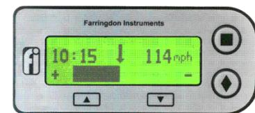
As soon as a faster lap is recorded, this is then taken as new standard against which to compare the current lap. To allow driver training where an instructor sets the best lap for the pupil to work towards, the best lap is held in non volatile memory (memory that remembers even when there is no power) and has to be manually reset to be removed. So power can be removed from the system between sessions without losing the instructor's "target" lap.
