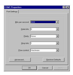
4 Click OK. The next dialogue box sets the serial line characteristics. It should be as shown below - 9600 bits per second, 8 bit data, no parity and 1 stop bit:
