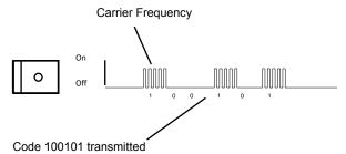
There are two ways in which this form of communication can be interrupted, first, by any light source strong enough to saturate the receiver - for example - the sun or another more powerful IR source - and second, other transmissions using the same carrier frequency.
