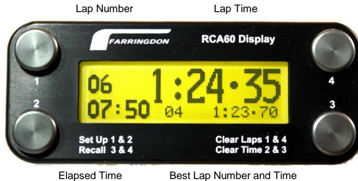
**The RCA60 Series of Lap Timers are designed for cars, bikes and karts. There are four versions of the lap timer, the RCA60, RCA61, RCA65 and the RCA66. The RCA65 and RCA66 have the new Delta Time Function.**
